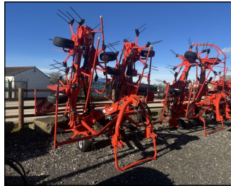
New Kuhn GF 8703 8 rotor tedder, 8.7m, hydraulic folding, hydraulic oblique, mech stabiliser, wheel & tine deflectors. £POA
