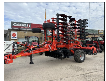
New Kuhn Optimer L 6000, 6m disc cultivator, following harrow, 600mm roller, hydra brakes, depth control wheels. £POA
