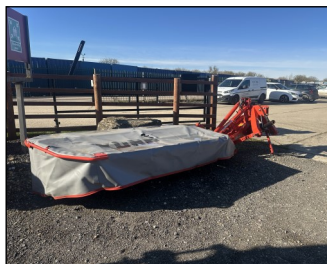
New Kuhn GMD 280 rear mower, 2.8m working width, hydraulic lift/fold, spring suspension. £POA
