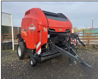
New Kuhn VB 3260 OPTICUT, integral rotor with Hardox tines, 14 selectable knives, drop floor, ISOBUS control. £POA
